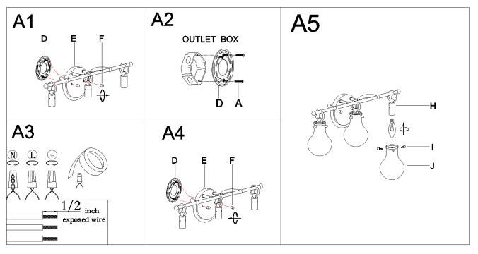
Step A1: Unscrew the studs(F) from the back plate(E) then gently remove the mounting plate (D). Step A2: Secure mounting plate (D) to outlet box with mounting screws (A).
