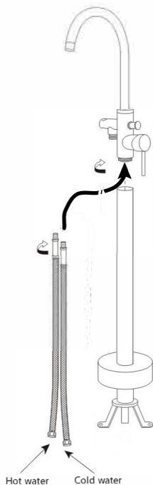
3. Install the flexible hoses to the valve body.
