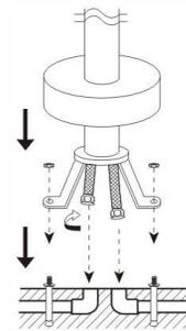
5. Tighten the screws to the permanent seat on the ground. Screw the flexible hoses into the outlet of the hot and cold water pipes.
