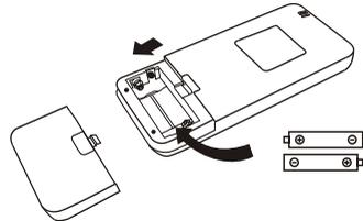
⚠ For some models, each time when insert the batteries in the remote controller for the first time, you can set the Cooling only or Heating pump control type. As soon as you insert the batteries, turn off the remote controller, and operate as below.
