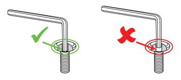
If the hex key is not fully inside the notch, the hex key could slip out, causing damage to the bolt head. Repeated hex key slipping will cause the notch to become rounded, making it difficult or impossible to tighten the bolt with the hex key.
