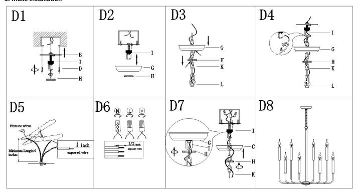
Step D1: .Attach single bar (B) to outlet box with mounting screw (D). The side of single bar marked "GND" must face out Unscrew threaded ring (H) from collar loop (I)
