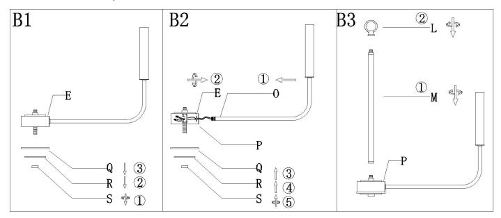
Sept B1:Unscrew the finial (S) from fixture body (P)then remove the bottom trim (R)and lid (Q) from fixture body (E)
