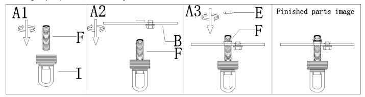
Step A1:Thread the nipple(F) into the screw collar loop (I)until snug
