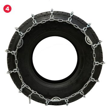
If you are in a safe situation, drive 150-300 feet and let the chain center on the tire. Check for tightness and make sure the chain is centered like the picture shows. Often times you can close the last cam at this point to get a good fit, or you might need to undo the cams and get one more link tighter on the outside speed hook. Then re-tighten cams for proper fitment. Multi-arm adjuster recommended.
