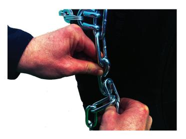
Start by hooking the speed hook on the inside of the tire, and then fasten the hook on the outside of the tire. Try and have them even or close to the same link on the inside as the outside, so one side chain isn't pulling more than the other. Try to get the inside and outside side chain as tight as possible.
