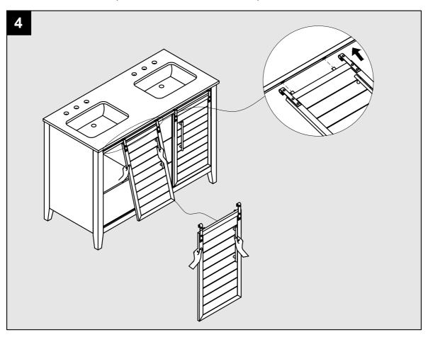
Note: In case replacing the slider sub-assembly, untighten the bolts with Allen wrench (not included).
