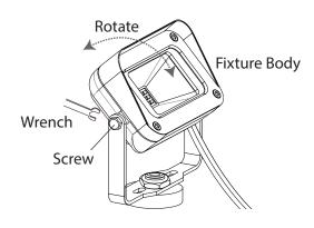
Adjust the fixture body to the desired orientation and tighten the screws with the wrench.
