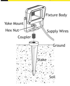
Thread the coupler onto the stake. Place the yoke mount of the fixture body over the coupler and secure with the hex nut. Hand tighten until snug.
