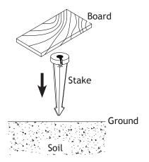
Determine the desired location for mounting the stake. Hammer the stake into the ground until flange of stake is flush to grade. To avoid damage to the stake, place a board on top of the stake while hammering.
