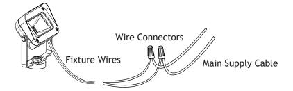
Strip both leads from the fixture wires. Using two UL listed wire connectors (sold separately), connect the leads from the fixture wires to the main supply cable leads.
