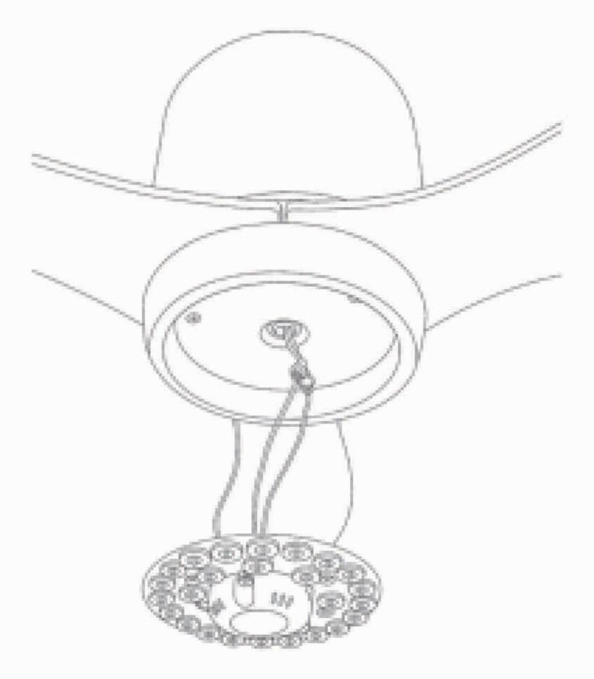
2.After locking the lamp kit, insert the LED wire ends.
