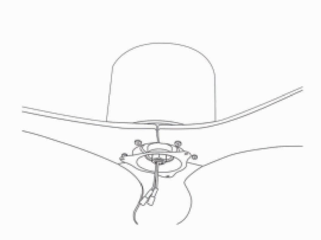
1.After locking the blade, install the lamp kit
