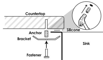
**Option 1.** Insert anchors under the countertop on the drilled holes, so they are ready to fasten the sink flange. Anchors should be inserted with a hammer until flush.
