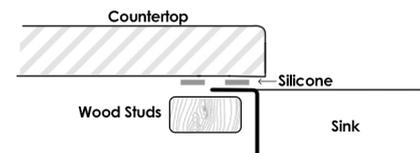
**Option 2.** Alternatively wood studs combined with silicone caulk can be used to hold sink against countertop without using mounting brackets.
