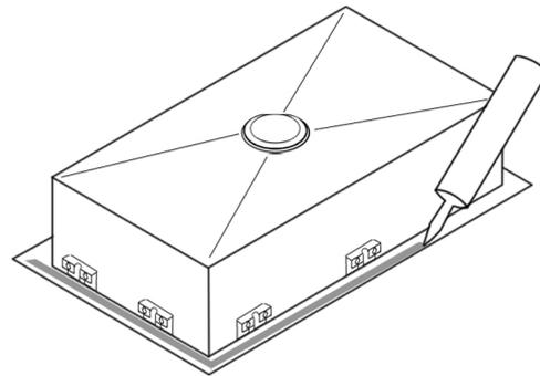
Clean sink flange and area surrounding the cut-out area of countertop, making sure that the area is smooth and free of debris. Apply continuous bead of silicone.
