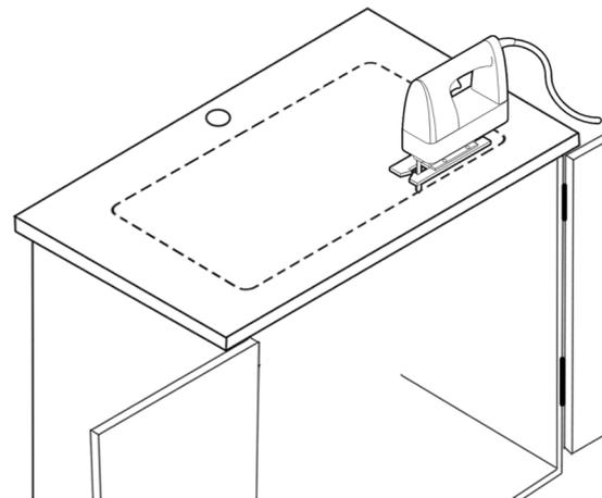
Trace the outline of the template and cut countertop according to templated outline using appropriate cutting tools. Template is for guide only. Use physical sink to ensure accurate cut-out opening. It is recommended to use the actual sink dimensions to ensure the most accurate cut out. Drawing or template are for reference.
