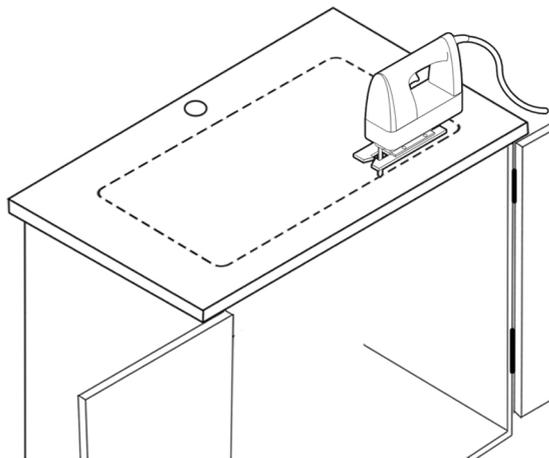
Trace the outline of the template and cut countertop according to templated outline using appropriate cutting tools. Template is for guide only. Use physical sink to ensure accurate cut-out opening.
