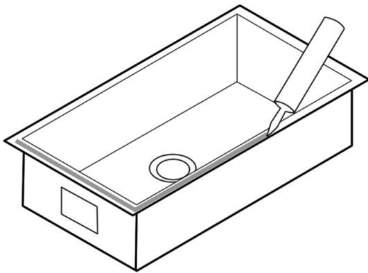
Clean sink flange and underside of cut-out area of countertop, making sure that the area is smooth and free of debris. Apply continuous bead of silicone caulk evenly on top of sink flange.
