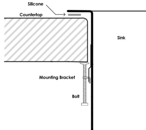
Insert mounting brackets on the side of the outer walls of the sinks on the slots provided.
