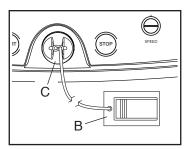
will light. IMPORTANT: In an emergency, the key can be pulled from the console, causing the walking belt to slow to a stop. Test the clip by carefully taking a few steps backward; if the key is not pulled from the console, adjust the position of the clip.
