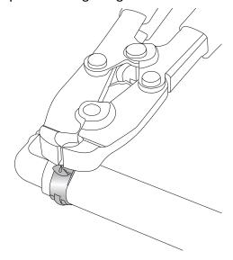
3. Cut through and remove clamp
