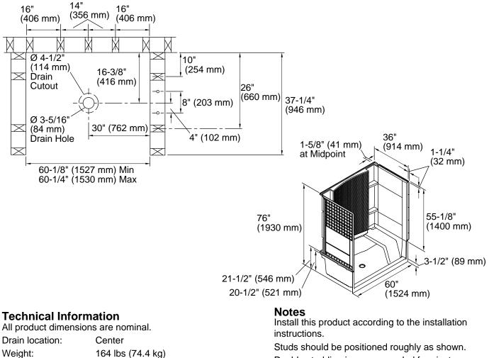
Studs should be positioned roughly as shown. Double studding is recommended for pivot shower door installations.
