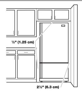
To ensure proper ventilation for your refrigerator, allow for a ½" (1.25 cm) space on each side and at the top. Allow at least 1" (2.54 cm) between back of cabinet and the wall. If your refrigerator has an ice maker, make sure you leave some extra space at the back for the water line connections.
