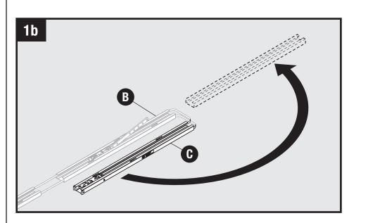
Slide the door end rail section (C) to correct position.
