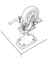
Install 4pcs 4-inch wheels from the bottom. Place spacers, spring washers and screws into each hole. Tighten the screws and fix. Note: The wheels are divided into universal wheels and fixed wheels. 2 PCS universal wheels will be under one side of the handle.Install 4pcs 4-inch wheels from the bottom. Place spacers, spring washers and screws into each hole. Tighten the screws and fix.
