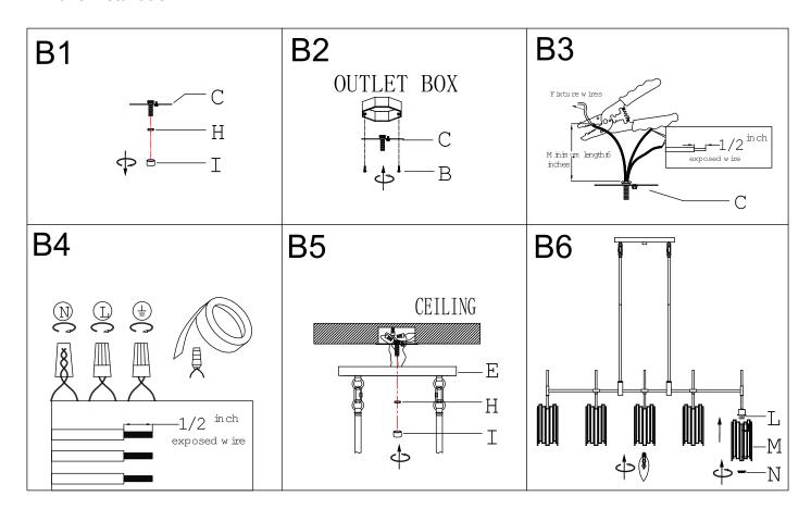
Step B1 » Unscrew hex nut (H) and cap nut (I) from single bar (C).
