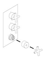
5. To install the hand shower's water supply elbow, thread it onto the prepared 1/2" NPT pipe nipple. Apply thread sealant or plumber's tape to the threads before tightening. Be sure to use the decorative escutcheon to conceal the rough-in.
