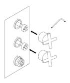
4. To install the temperature control handle, loosen the set screw and remove the handle from the handle base. Attach the handle base to the center stem using the provided screw. Tighten with a Phillip's screwdriver, then reattach the handle.
