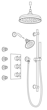
12. Turn the main water supply back on, and test the completed shower system. Ensure that there are no leaks and that all functions are working properly.
