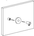
6. Determine a location to mount the hand shower's slide bar. Temporarily install the mounting brackets onto the bar, and hold the bar against the wall at its desired mounting location. Use a level to ensure that the slide bar is straight, then mark the locations of the mounting brackets by outlining them with a pencil. Remove the bar, then attach the brackets to the wall using the provided anchors and screws.
