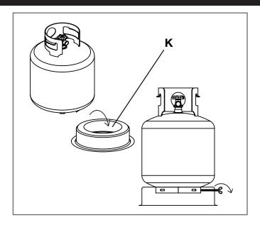
8. Turn the cylinder valve on the tank clockwise to close the propane tank. Attach the preassembled regulator from the firebowl body (C) to the cylinder valve by turning the regulator coupling nut clockwise. Make sure it is fastened securely and tighten connections by hand only.
