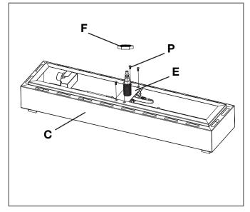
**4.** Insert the threaded post into the umbrella hole on the tabletop so that the bottom of the firebowl body (C) sits flush on the tabletop. Secure the firebowl body (C) to the table by screwing the fixing nut (F) onto the threaded post underneath the tabletop. Be sure to tighten securely.
