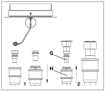
**6.** Pull back and hold the collar on the female end of the quick disconnect connection (H) coupling. Insert the Quick Disconnect male end (G) fully into the coupling and then release the collar.
