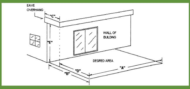
Measure the width of the area to covered ("A"). Round to the nearest even foot increment. "A" will be the total width of the patio cover.
