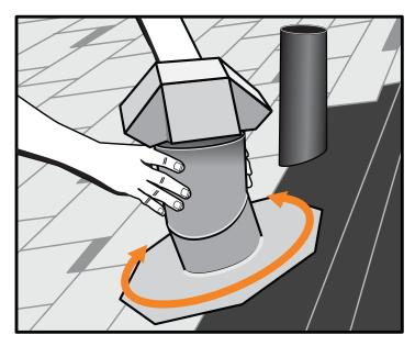
1. Set **TOTAL JACK™** down, flat on the surface of the roof, next to the pipe you are ventilating. Rotate the octagonal base flange to achieve a vertical, upright position.
