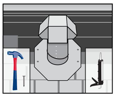
**3**. Secure octagonal flange with fasteners as approved by your local building code. Add a dab of caulking to seal the fasteners Install remaining shingles in accordance with manufacturer's specification.
