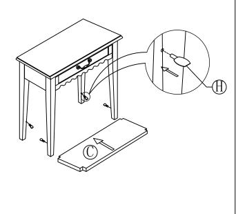
Step 3 Now tighten the bolts in Step 1 and put the drawer back into the table.
