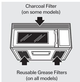
The vent fan has two metal reusable grease filters.
