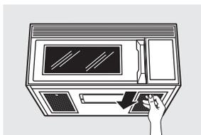
**To remove**, slide them to the side using the tab. Pull them down and out.
