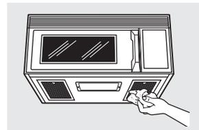
Clean off the grease and dust on the bottom often. Use a solution of warm water and detergent.
