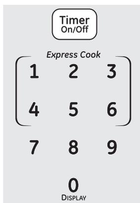
Timer On/Off operates as a minute timer and can be used at any time, even when the oven is operating.
