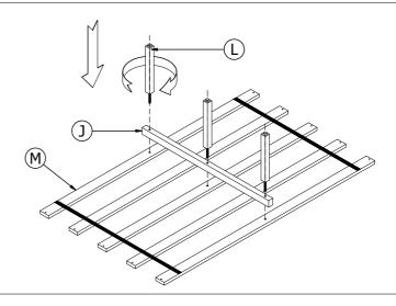
Step 6. Set Slat roll(M), link pre-wire up. Next, place the Long center supprot slats(K), align the drill holes.
