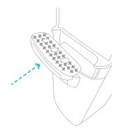
3. Gently pull the drip tray toward you to release it. Once it has been released you can remove the drip tray from the door of the cooler to empty it.
