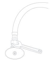
3. Connect the Metal Adapter with Valve between the cold water supply line and cold water valve.
