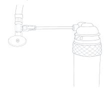
2. Take the open end of the PE Tubing that is now connected to your water supply and insert it into the left inlet hole on the Filter Flushing Adapter in the direction of the arrow.
