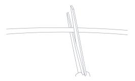
3. Insert each cut end of the existing ¼" Tubing into one of the holes of the Three Way Plastic Adapter.
