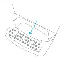
2. To remove the drip tray, place your fingers in the grid of thte drip tray with one hand and <u>hold the door</u> of the cooler shut with the other.
