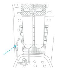
5. After installation of the water line and filter is complete, plug the power cord into a grounded wall outlet and begin to use the machine. Please allow the machine about 10-15 minutes for the water to fill in the tanks before use. Continue on for instructions on usage.
