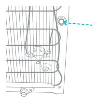
3. Turn the Valve for the water source back on (the on position is parallel to the PE Tubing).
