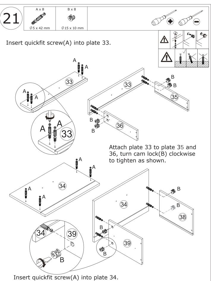
Insert quickfit screw(A) into plate 34. Attach plate 34 to plate 38 and 39, turn cam lock(B) clockwise to tighten as shown.
