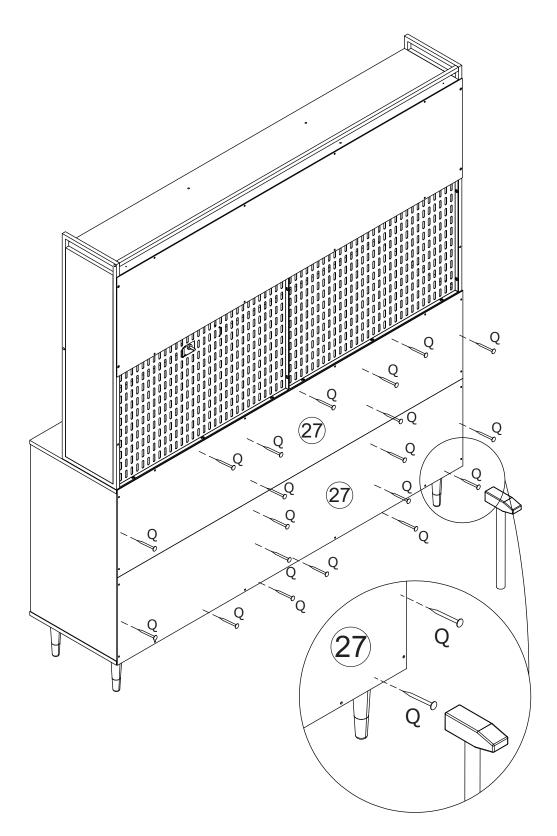
Reinforce back plate 27 using nail(Q) as shown.
