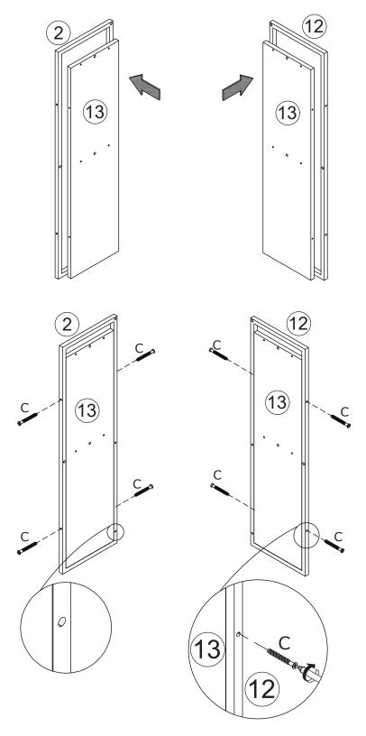
Fix plate 13 to iron stand 2 and 12 respectively with screw(C) as shown.
