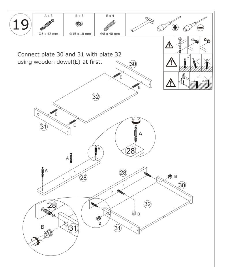
Insert quickfit screw(A) into plate 28 as shown. Attach plate 28 to plate 30,31 and 32, turn cam lock(B) clockwise to tighten as shown.
