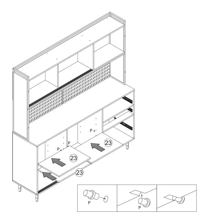
Insert part(P) into plate 19, 21 and 22, then place shelf 23 in as shown.
