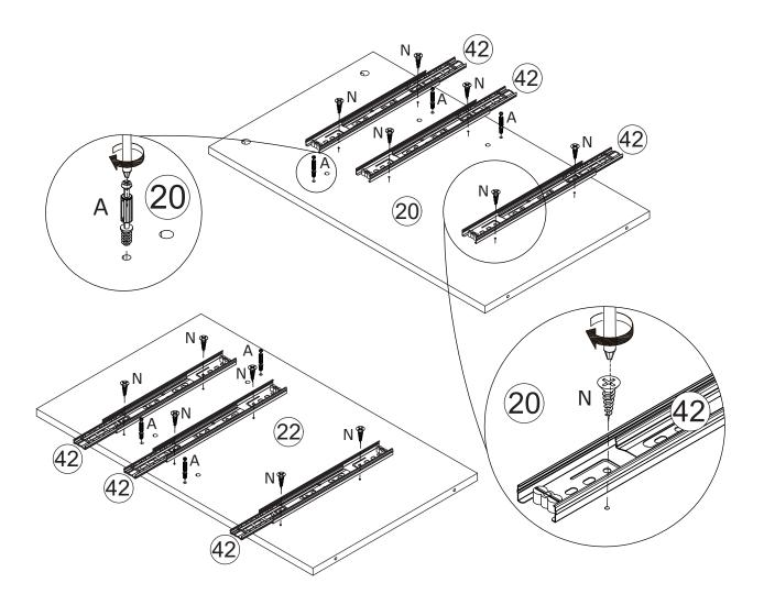
Fix slide rail 42 to plate 20 and 22 with screw(N) as shown Insert quickfit screw(A) into plate 22 and 20 as shown.
