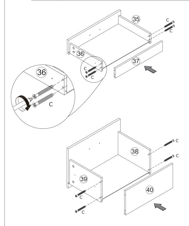
Fix plate 37 to plate 35 and 36 with screw(C) as shown. Fix plate 40 to plate 38 and 39 with screw(C) as shown.
