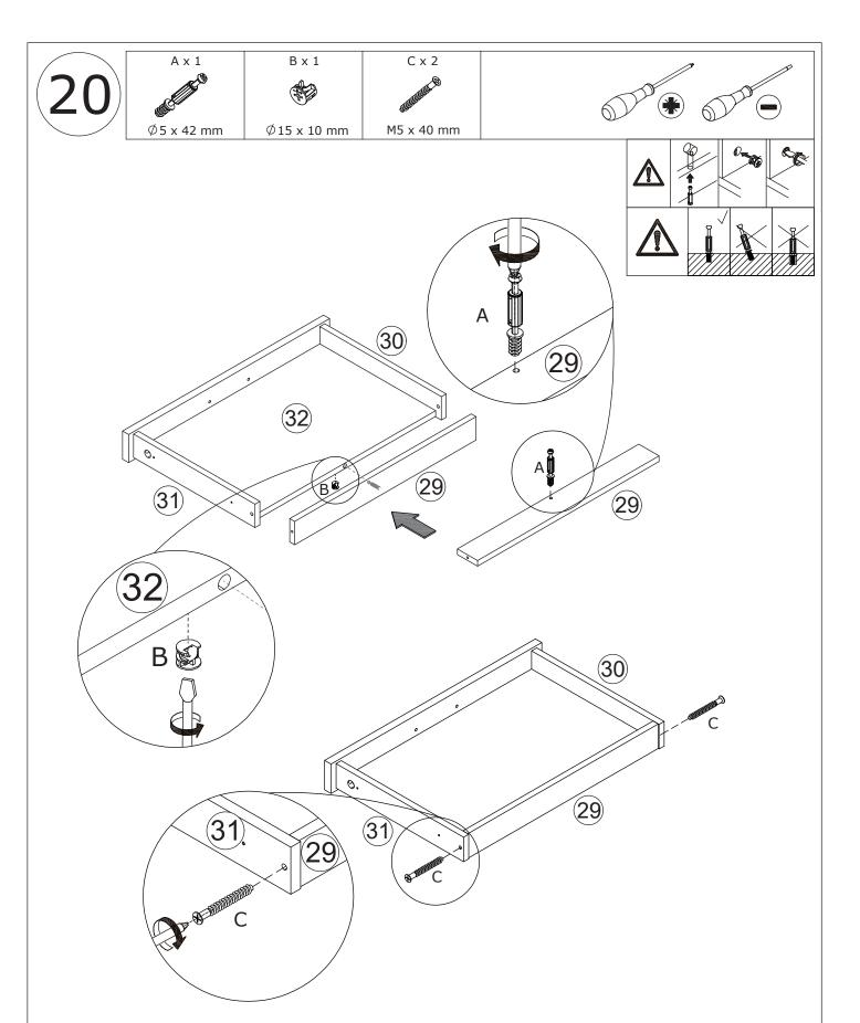
Insert quickfit screw(A) into plate 29, attach to plate 32 and turn cam lock(B) clockwise to tighten.
