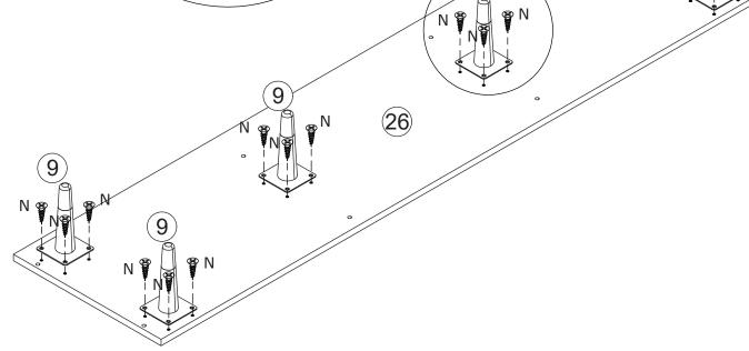
Fix leg 9 to plate 26 with screw(N) as shown.
