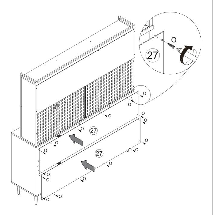
Fix back plate 27 to the cabinet with screw(O) as shown.
