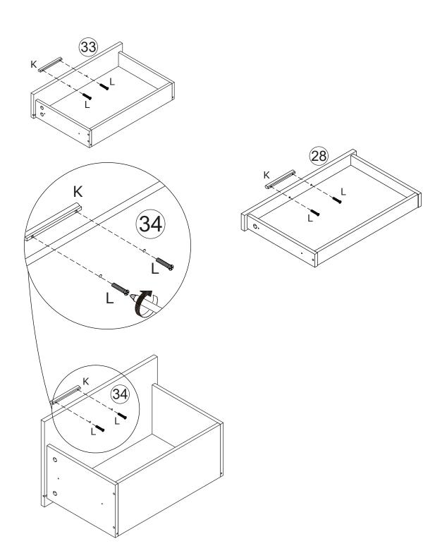
Fix handle(K) to drawer face with screw(L) as shown.
