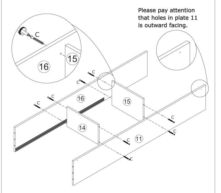
Fix plate 11 and 16 to plate 14 and 15 with screw(C) as shown.
