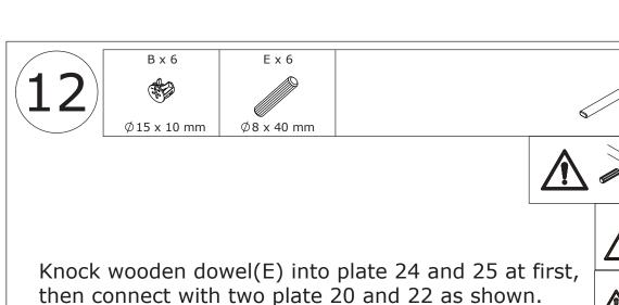
Knock wooden dowel(E) into plate 24 and 25 at first, then connect with two plate 20 and 22 as shown. Add cam lock(B) into plate 24,25 and turn clockwise to tighten as shown.
