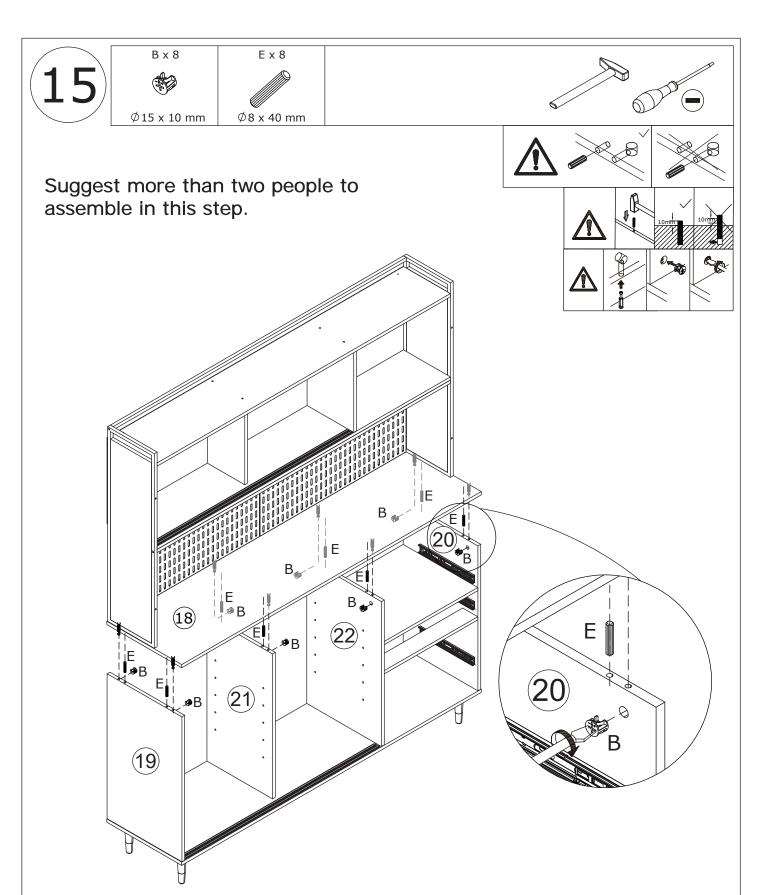
Knock wooden dowel(E) into plate 19, 21, 22 and 20 at first, then connect the two components as shown.
