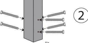
Slide the surface mount post onto the base plate. Using the 6 bolts included with the base plate, secure the post to the base plate by tightening the bolts. The top of your post should now be 30 to 34 inches above street level.
