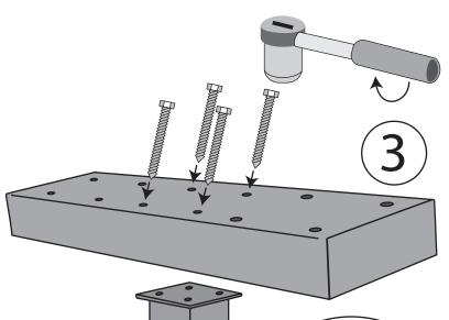
Center the spreader bar on the post and secure the spreader bar by inserting and tightening the 4 bolts included.
