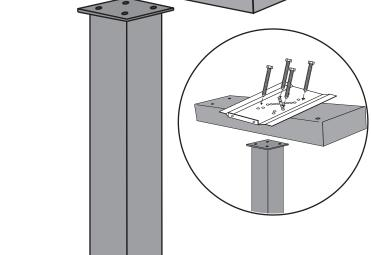
If you're installing a mailboss with a mounting plate on a 3 box spreader install the 4 bolts through the mounting plate first, then through the spreader bar, and lastly through the post to secure them.
