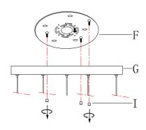
4 » Carefully pass the supply wires from the outlet box through mounting plate (F).
