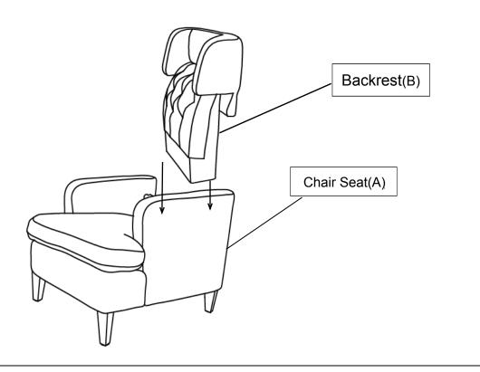
Position yourself behind the chair. Place Chair Backrest(B) into the Chair Seat(A). While tilting the Chair Backrest(B) slightly forward. Then gently pull the Chair Backrest(B) towards you while pushing it down all the way into the Chair Seat (A) slot located to the rear of the Chair Seat(A). (as marked by the arrow above).
