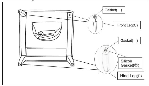
Install the first Front Leg(C) into the Chair Seat(A) by placing one Gasket( ) onto the threaded stem.
