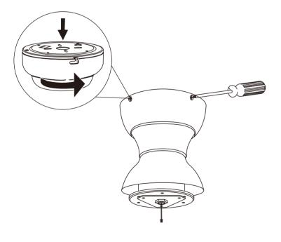
3. Attach the housing to the mounting plate, aligning the keyhole slots on the housing with the screws on the mounting plate and twist clockwise until tight. Tighten 4 screws.
