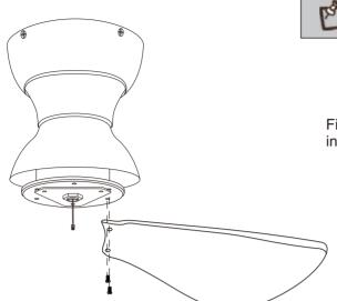
NOTE: Your fan features revolutionary advancements for quick and easy blade installation. Including an alignment post and captive blade arm screws.
