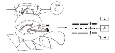
2. Hang the ceiling fan light on the hook of the mounting bracket and use a wire connector for wiring.
