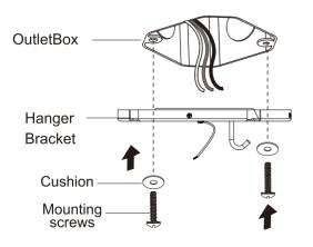
Before installing this fan make sure the outlet box is properly installed to the house structure.
