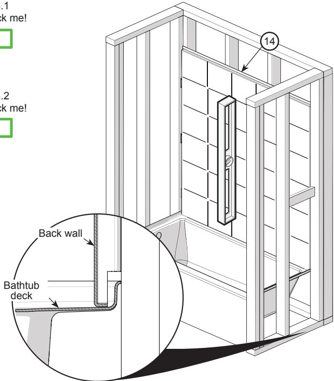
With a 1/8" bit, drill holes in the back wall fastening flange (14) at the top aligned with each stud. **Only pre-drill the flange not the studs.** Then, secure the back wall (14) with **one #8 x 1 1/4" screw** (not included) in one of the pre-drilled holes.
