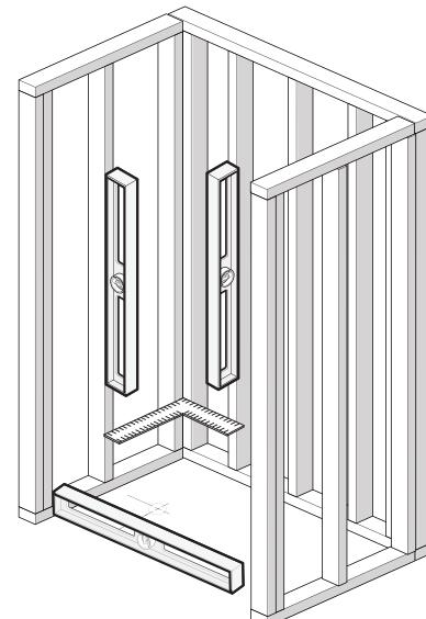
Cut out an approximate 6" x 6" opening around the drain center outlined by measurements C and D. See image to the right and the chart above. We recommend that a plumber completes the drain pipe connection.
