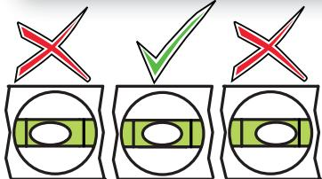
Plumbing the back wall is critical for alignment of the side walls
