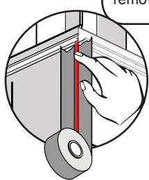
Apply masking tape on both sides of the joint where you will run a bead of silicone. Apply the silicone, smooth with a wet finger then remove the masking tape.
