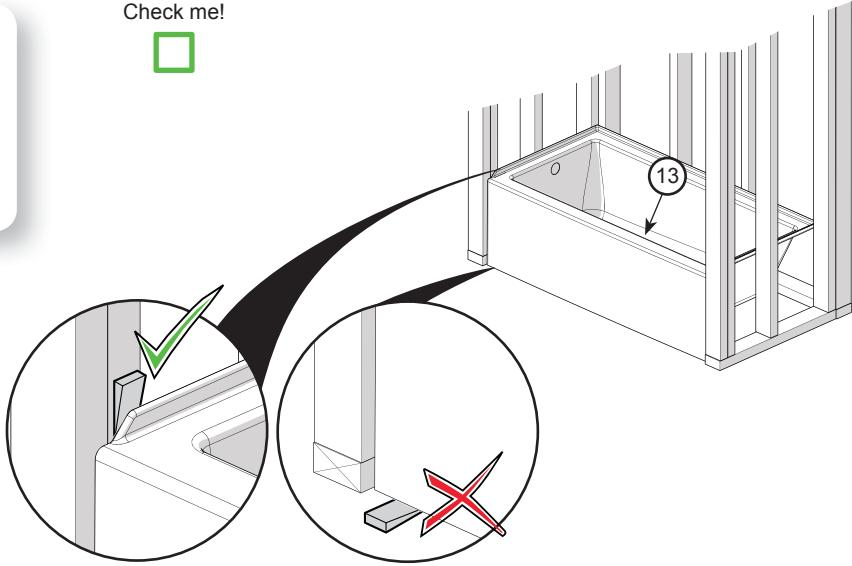
With a 1/8" bit, drill holes in the bathtub fastening flange then secure the bathtub to all the wall studs with #8 x 1 1/4 " screws (not included). **Only pre-drill the flange not the studs.**
