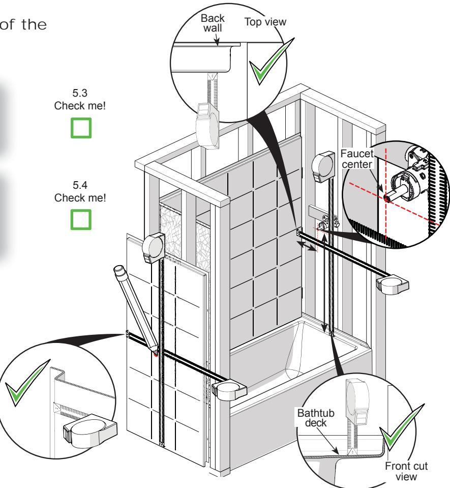
Drill a hole from front for the faucets at the previously marked positions. Pre-drill the hole with the  $\frac{1}{8}$ " drill bit. The hole saw size is determined by the faucet type; refer to the faucet installation manual for hole saw size.
