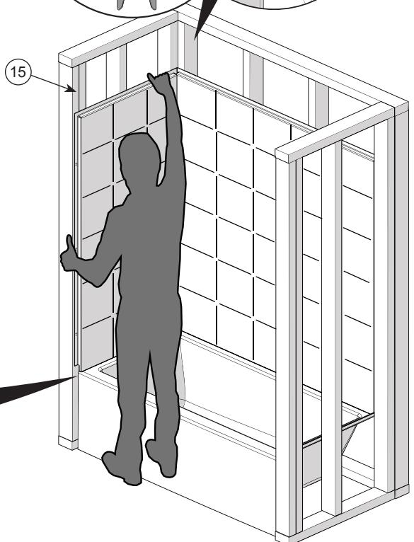
With a 1/8" bit, drill holes in the side wall fastening flange (15) at the top aligned with each stud. **Only pre-drill the flange not the studs.** Then, secure the side wall (15) with **one #8 x 1 3/4"** screw (not included) in one of the pre-drilled holes.
