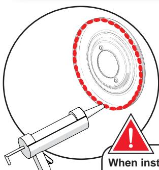
When installing the faucet faceplate or any other component, be sure to silicone the outer edge.
