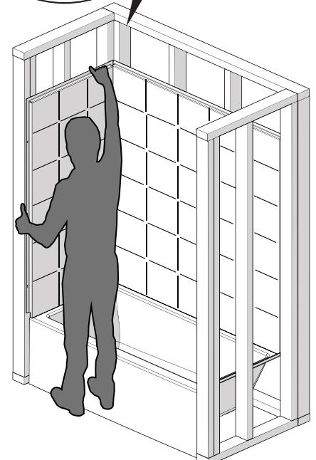
Install the side wall (15) with the faucet hole. Lift the wall approximately 3 inches above the deck of the bathtub, push it completely against the back wall then slide the side wall into position.
