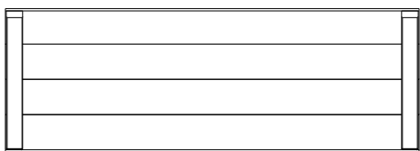
RP3 | PEAK ROOF PANEL - W2A02652 (1) | 1 5/8"x20 5/8"x59" (42x524x1499)
