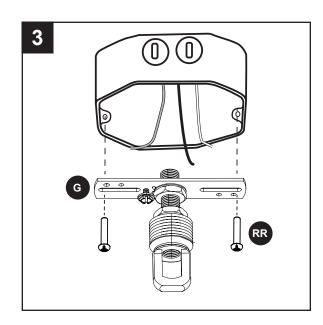
4. Loosen the ground screw (K) preassembled to mounting bracket (G) and wrap bare/green supply wire around the ground screw. Retighten the ground screw (K).
