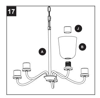
18. Insert E26-base bulbs (not included) into the sockets of the fixture (A).
