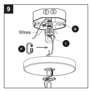
10. Twist nut to close connecting links (F) at each end of chain (D).
