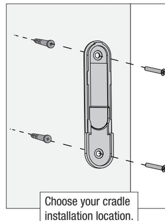
*If you are installing into drywall, drill two 9/64 width holes using the cradle bracket as a guide. Gently hammer the included drywall anchors into the pre-drilled holes.*
