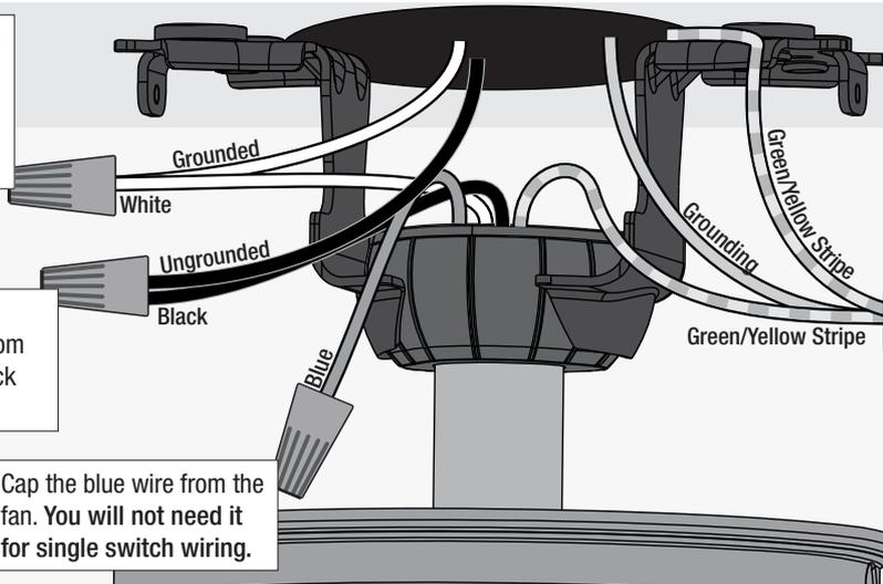
Connect the three grounding wires (green, green/yellow stripe, or bare copper) coming from the ceiling, downrod, and hanging bracket.
