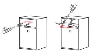
2 Using the template found on the reverse side, carefully arrange and mark the two top holes levelly and about 130cm to 165cm above the floor, or according to your preference, then mark the bottom two holes.
