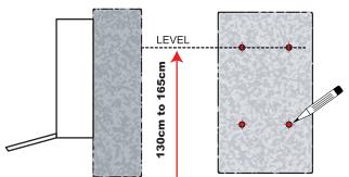
**3** Using the 4mm drill bit provided, create four pilot holes at least 10mm deeper than screws provided, or about 40mm deep. If the material is unusually hard you may need to use a rotary impact drill rather than a standard drill to make the holes. Call
