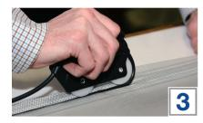
Using the spline tool, roll the fabric into the screen frame groove holding fabric straight while rolling. The spline should be pressed securely in the groove and in each frame corner. It may be necessary to push the spline into each corner using the utility knife or a screwdriver.
