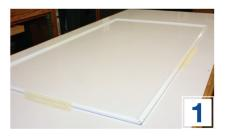
Place screen frame on a flat surface. Remove any existing spline. Tape outside edges of frame to the surface. Do not tape over the spline groove.
