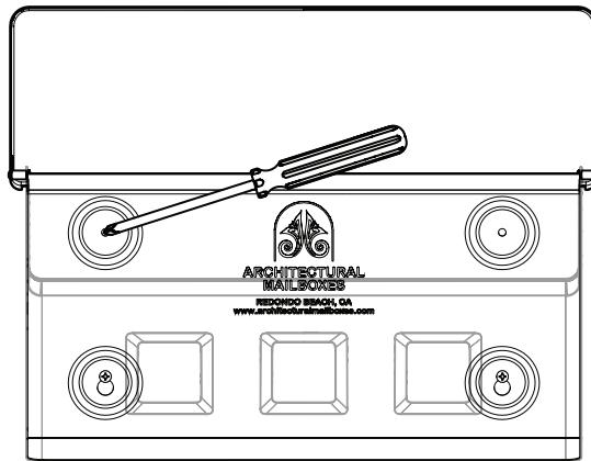
**5** While the mailbox is hanging on the bottom screws, insert the remaining two screws into the top holes and secure with a screwdriver.
