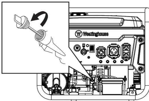
2. Using the supplied funnel and oil, add oil into oil filler neck.
