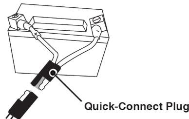
**Note:** The generator is equipped with a battery charging feature. Once the engine is running, a small charge will slowly recharge the battery.
