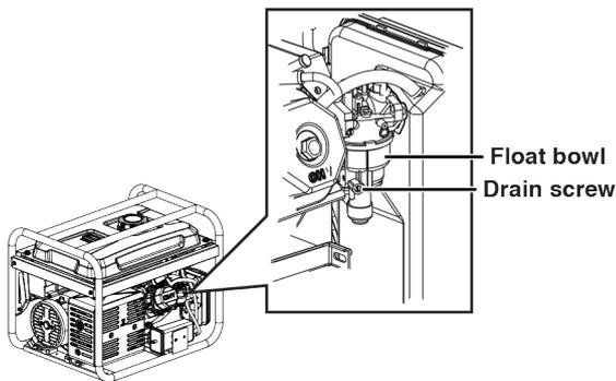
3. Place an appropriate gasoline container under the drain screw to catch the drained fuel.
