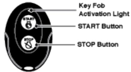
4. Push and hold the START button on the key fob until the START/STOP button illumination turns OFF. Release the button. The START/STOP button will illuminate after the button is released.
