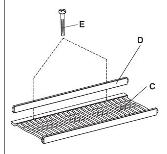
Attach the apron (D) into bottom of seat (C) and secure using 2 1/4" bolts (E).
