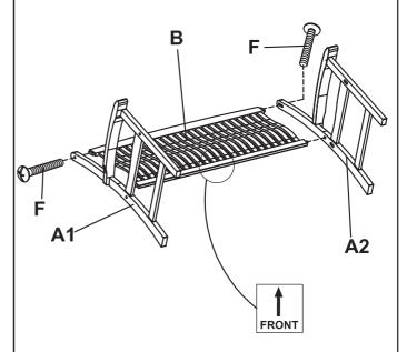
Attach right and left side frames (A1 & A2) into back support (B). Secure using 1" bolts (F).
