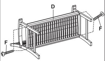
Next, attach the pre-assembled seat into right and left side frames (A1 & A2). (The seat with apron must be attached in front). Secure seat using 1" bolts (F) as shown. Tighten all bolts using screwdriver.
