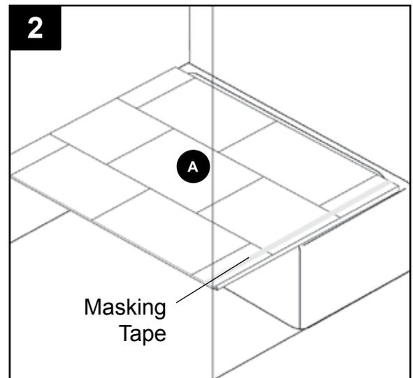
3. If needed, place 1/16 in. thick shims (not included) at the base of the lower back panel's (A) installation site. Trial fit the lower back panel (A) on the shims and use a sanding block if any fine adjustments are needed. Remove lower back panel (A) from wall and clean the back of the lower back panel (A), the wall board and any other area that will be in contact with the silicone (L) with denatured alcohol and a clean rag (both not included).
