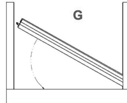
**3)** Measure the distance from wall to wall across the top of the jambs. Cut the ZTE2601A Header (#8) to that dimension minus -1/16". Slide the header down over the top of the wall jambs. The header does not need to be secured with screws. **(H)**
