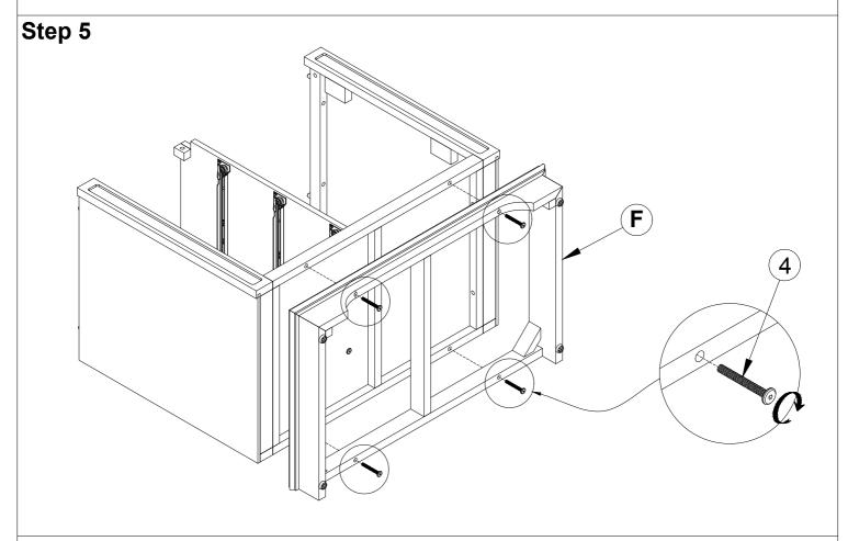
Insert Base frame (F) and Step 4 with Bolt M6x50 (4).
