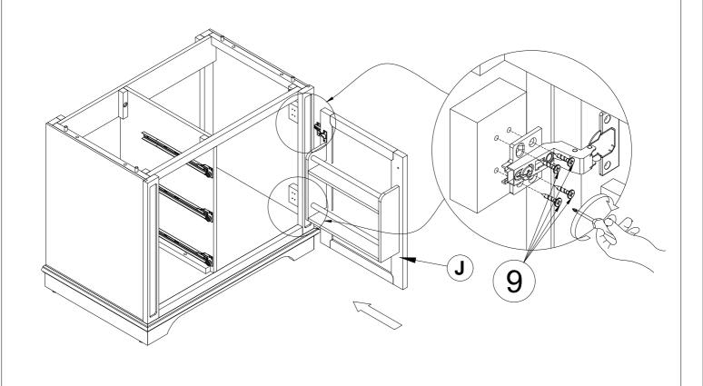
Insert Right door (J) and Step 7 with Screws M4x15 (9).
