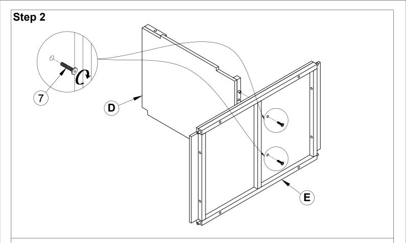
Insert Partition frame (D) and Bottom frame (E) with Bolt M6x25 (7).
