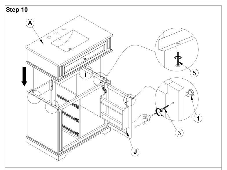
Insert Top (A) and Step 9 with Bolt M6x40 (5).
