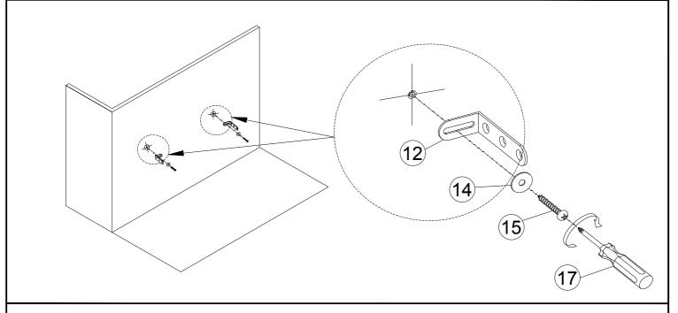
C: Affix the L-shaped Metal Bracket (12) to the wall.
