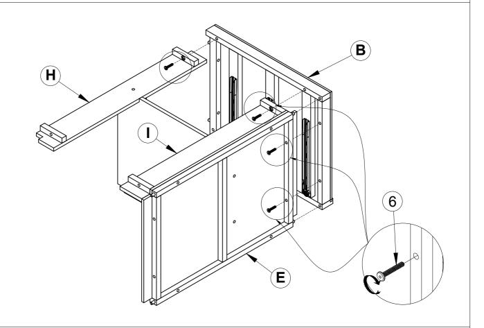
Insert Left side frame (B), Bottom frame (E), Rear top bar (H) and Rear bottom bar (I) with Bolt M6x30 (6).
