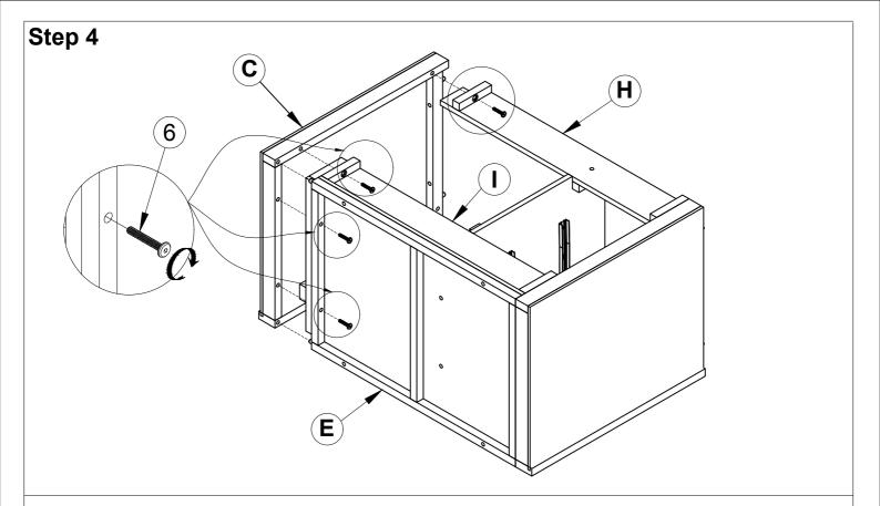
Insert Right side frame (C), Bottom frame (E), Rear top bar (H) and Rear bottom bar (I) with Bolt M6x30 (6).
