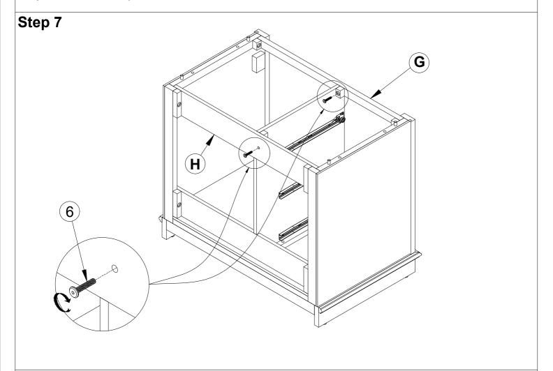
Insert Front cross bar (G), Rear top bar (H) and Step 6 with Bolt M6x30 (6).
