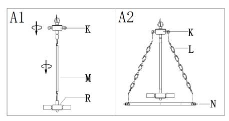
Step A1: Slip stem (M) over the wires and then thread it into the top of lower fixture loop assembly (R).
