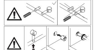
Attach No.9 and No.10 plate to No.14 with wooden dowel(C) and then fix with screw (D) as shown.
