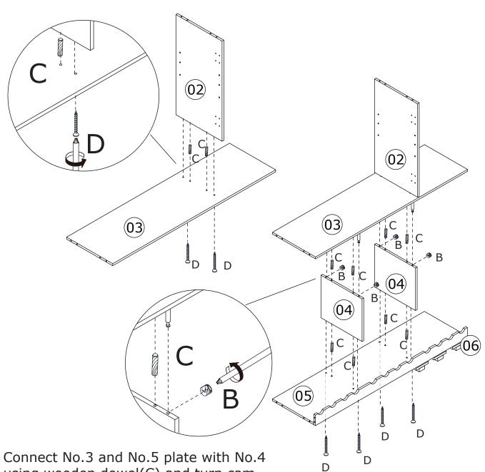
using wooden dowel(C) and turn cam lock(B) clockwise to tighten. Fix No.5 plate with screw(D) as shown.
