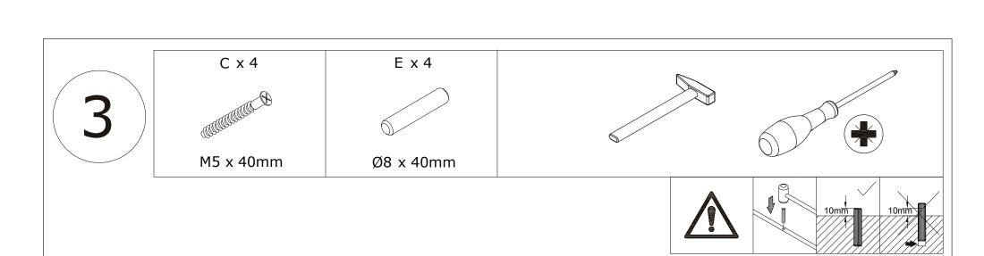
Connect No.3 and No.4 plate with No.2 using wooden dowel(E) and then fix with screw(C) as shown.
