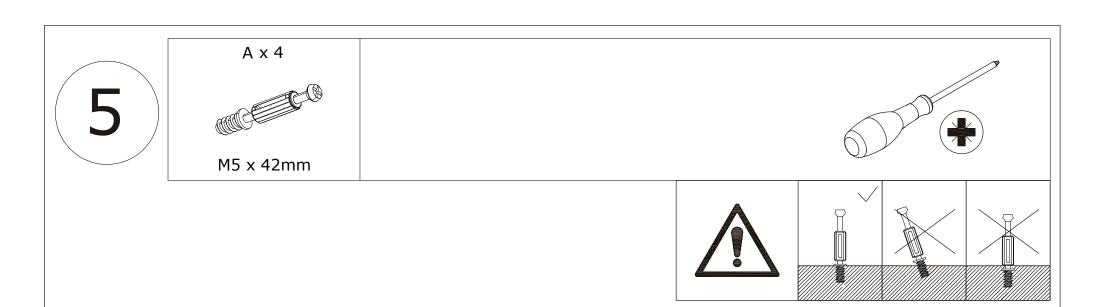
Insert quickfit screw(A) into corresponding holes in No.1 plate with a screwdriver as shown.
