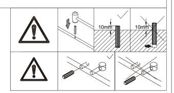
Slide No.5 plate into available grooves as shown. Knock wooden dowel(E) into No.3 and No.4 plate as shown.
