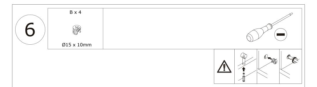
Cover No.1 plate to the top and turn cam lock(B) clockwise to tighten as shown.
