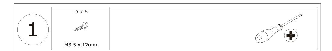
Separate glide into two parts at first. Fix No.11 slide rail to No.3 plate with screw(D) as shown.
