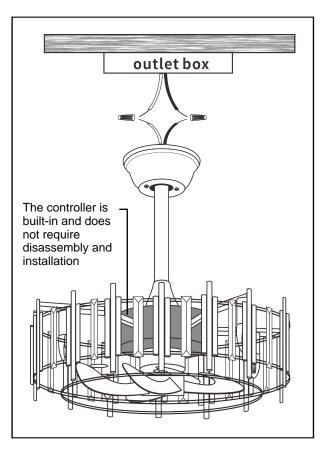
1. The wires of the motor are connected to the wires of the outlet box, and the black and white wires are not divided into positive and negative poles.
