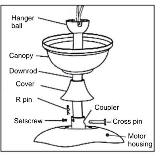
Loosen the two adjusting screws on the great. Fit connecting pin and screw into place. Make sure the alliance is tight.
