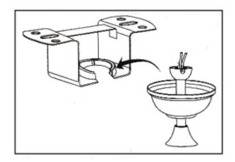
2.Carefully lift the fan joint and place it on the shaft of the hanger.Make sure that the hole of the bracket and the structure to be connected are aligned with the upper flange of the hanger.After wiring, press upward and twist to adjust the position of the screw hole to connect the canopy to the suspension bracket. Later,Connection of fixing screws.
