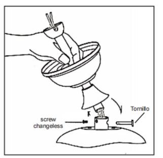
Remove connecting pin and unscrew it. Lead cable in through the lowering lever, considering these parts.
