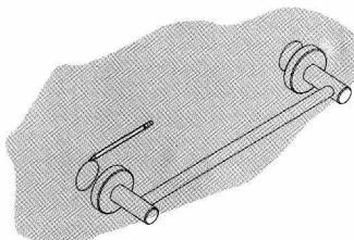
**2** Cover mounting bracket paper on marked circle base, mark 2 points according to paper holes to drill wall holes on each base side.
