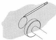
**2** Cover mounting bracket paper on marked circle base, mark 2 points according to paper holes to drill wall holes.
