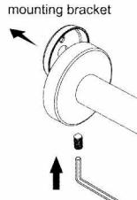
**6** Use screwdriver tighten the mounting bracket on wall stable.
