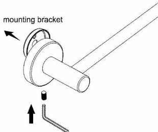
**6** Use screwdriver tighten the mounting bracket on wall stable.
