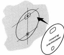
**3** Use 1/4 inch driller to drill holes on wall which you marked, the depth same as white anchor.
