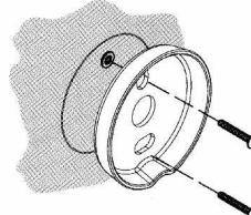
**7** Put the accessory onto mounting bracket and tighten the setting screw in bottom.
