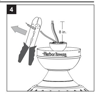
5. If you decided to cut back the lead wire in Step 4, strip 1/2 in. of insulation from the end of the white wire. Twist the stripped ends of each strand of wire within the insulation with pliers (not included). Repeat the step for black and blue wires.
