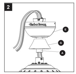
3. Slide the downrod (A) into the yoke of the motor assembly (H), align the holes, then re-install the downrod pin (B) and downrod clip (C). Secure with set screws (I) and slide the yoke cover (G) down until it rests on top of the motor assembly (H).
