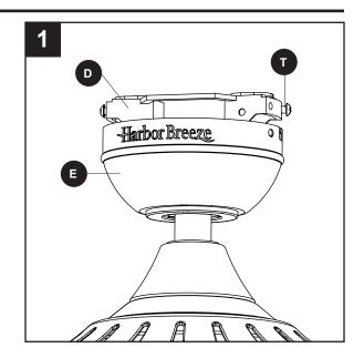
2. Secure the canopy (E) with the mounting bracket screws (T) previously removed (Step 4, page 8). Tighten all mounting bracket screws (T) securely.
