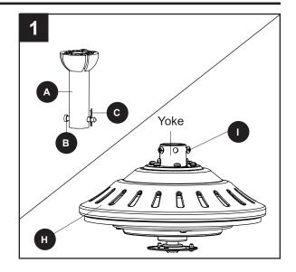
2. Insert the downrod (A) -- or a longer downrod, if required -- through the canopy (E) and yoke cover (G). Feed the wires from the motor assembly (H) through the downrod (A).
