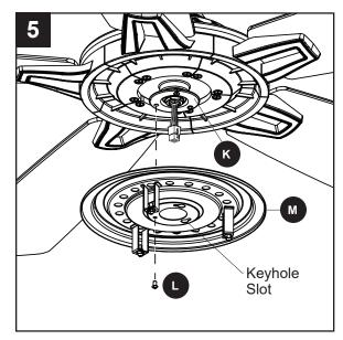
6. Remove one and loosen the other two light pan screws (N) from the underside of the light pan (M). Connect the 9-pin connector from the fitter plate (K) to the 9-pin connector from the light kit (O). Align the keyhole slots in the light kit (O) with the loosened screws in the light pan (M). Turn light kit (O) clockwise and replace the previously removed light pan screw (N). Tighten all screws.
