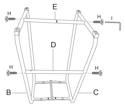
**STEP 3** Attach the Leg Frame (B&C) to the Seat (A) as shown in below diagram by using Allen Bolt (G) and Allen Wrench (I), **Please tighten the bolts to 90%.**
