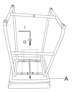
**STEP 4** In this step please make sure the chair legs are flat and all bolts are installed, then please tighten all bolts (F,G,H) to 100%. A few days after initial assembly, the product may acclimate to its new environment. Please ensure all bolts are still securely tightened.
