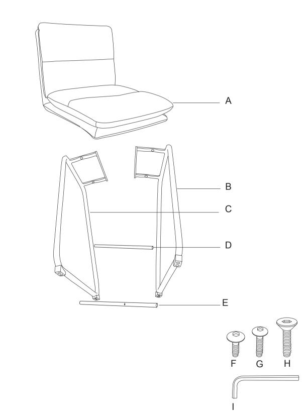
**STEP 1** Attach the Left Leg Frame (B) to the Right Leg Frame (C) as shown in below diagram by using Allen Bolt (F) and Allen Wrench (I), **Please tighten the bolts to 90%.**
