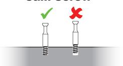
Use a screwdriver to tighten the cam screw until the shoulder is flush with the panel. Do not over-tighten or under-tighten.
