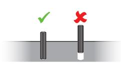
Install wood dowels by gently tapping them into the designated hole using a rubber mallet.
